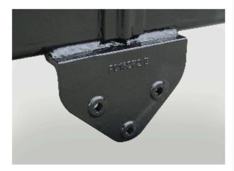
This hoist is easily installed on the trucks chassis' using extra heavy duty 4140 grade cast mounting brackets, with eight 1/2" and two 5/8" grade 8 bolts.
