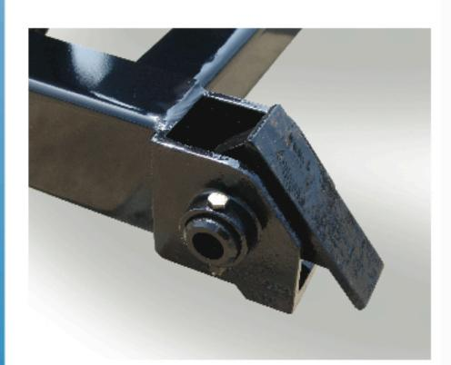
The hinges are cast 4140 grade steel to ensure durability. Adding to the ease of installation and durability, these hinges are welded directly to the body's longitudinals.
