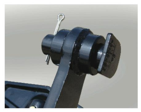
Shown is a U624A heavy duty lift arm. These arms easily attach directly to the body using 4140 grade, 1 1/2" hinge pins. The arms have easily accessible zerk grease fittings.
