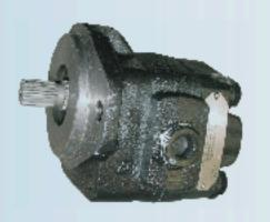
The P21 direct mount gear pump is bi-rotational with side and rear ports for versatility, thus eliminating the drive line for added safety and dependability. This pump has an S.A.E. "B" 2-bolt flange . 10 GPM @ 1200 RPM
